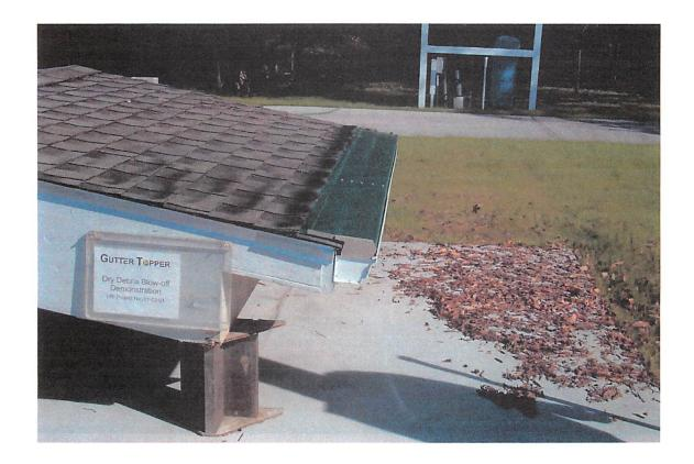
After Dry Debris Trapping Test
