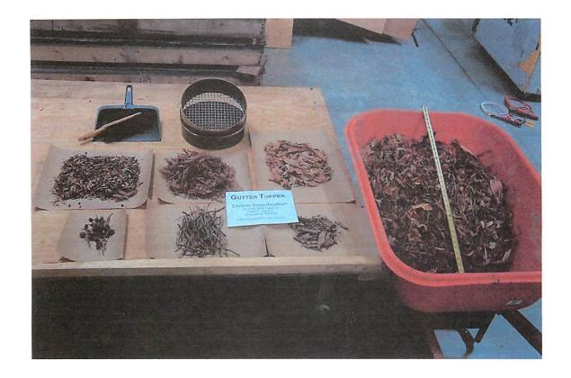
**Test Debris Quantification**
